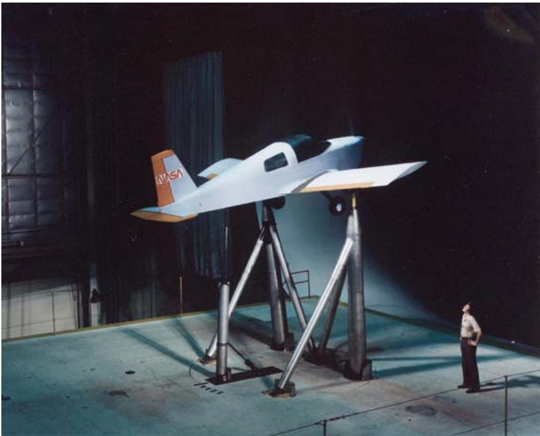
*Researcher Dale Satran inspecting full-scale powered model of AA-1 research aircraft during tests of automatic stall-prevention concepts in Langley 30- by 60-Foot (Full-Scale) Tunnel.*
