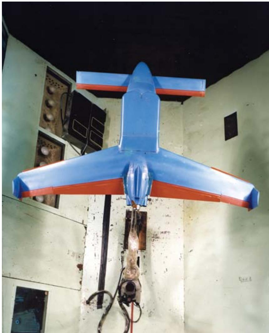
*Model of OMAC 300 in Langley 12-Foot Low-Speed Tunnel.
