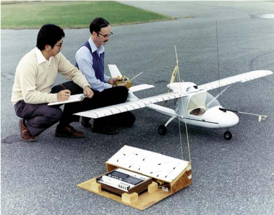
*Long Yip and David Robelen prepare radio-controlled model of DeVore Sunbird for flight tests.
