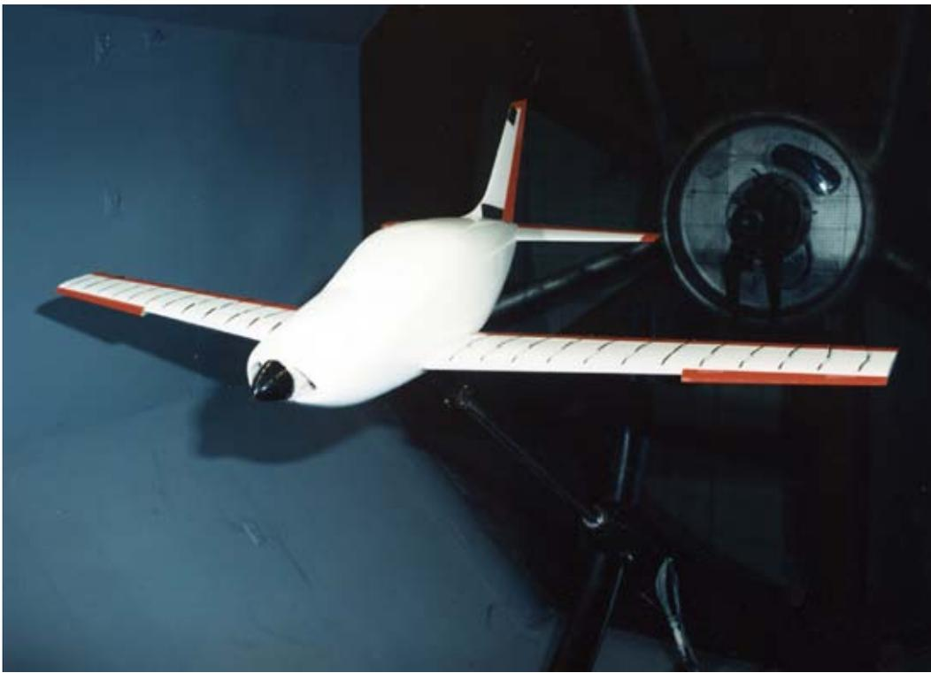
*Model of Questair Venture aircraft in Langley 12-Foot Low-Speed Tunnel during tests to develop spin-resistant wing configuration.*
