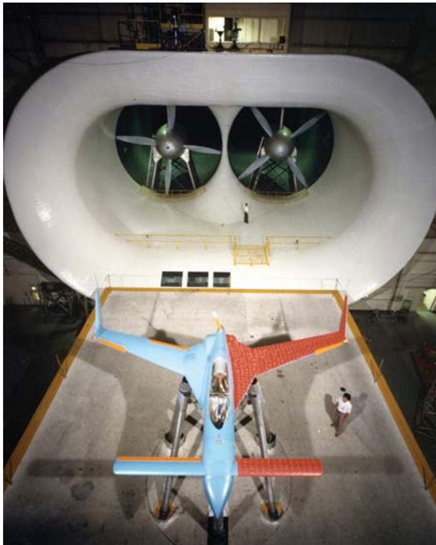
*Long Yip with full-scale model of Rutan VariEze aircraft in Langley 30- by 60-Foot Tunnel.
